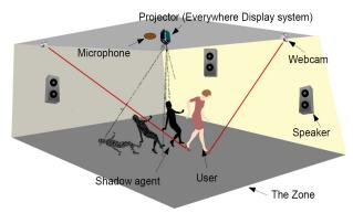
Figure 1. System's hardware components overview.
