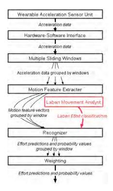
Figure 2. The EFFORTDETECT'S architecture. Components in red are active in the training phase
