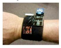
Figure 1. The Wearable Acceleration Unit
