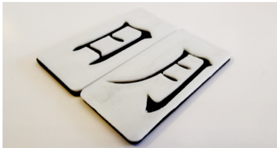
Figure 6: The 3D printing of the radical cards 日 (/ri4/, sun) and 月 (/yue4/, moon) in the size of 4*2*1cm. We printed out one white layer and one black layer and glued them together.
